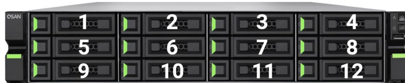
Figure 2-2 Disk Drive Numbering
