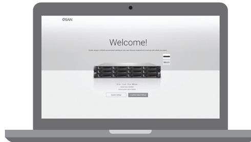
After all configurations are set up, the system will redirect your page to the new IP address you just set for the management port. Then you have to login with new admin password.
